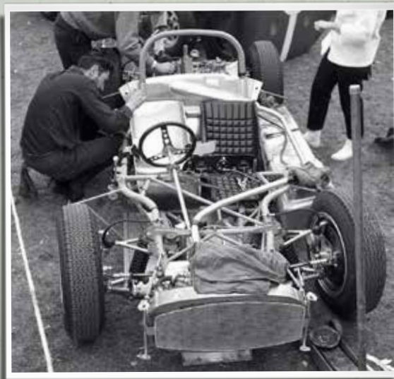
June 23, 1963 - SCCA Nationals, Road America, Elkhart Lake, USA - the 'curly-wurly' or 'plumber's bend' offset-drive 'Zerex Special' chassis form whose centre section would be replaced by the embryo McLaren team in 1964. © GPL
