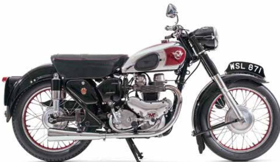
Announced in 1948, the Matchless G9 and equivalent AJS Model 20, while following the established pattern of British parallel twins, were unusual in having a third, central, crankshaft main bearing.
