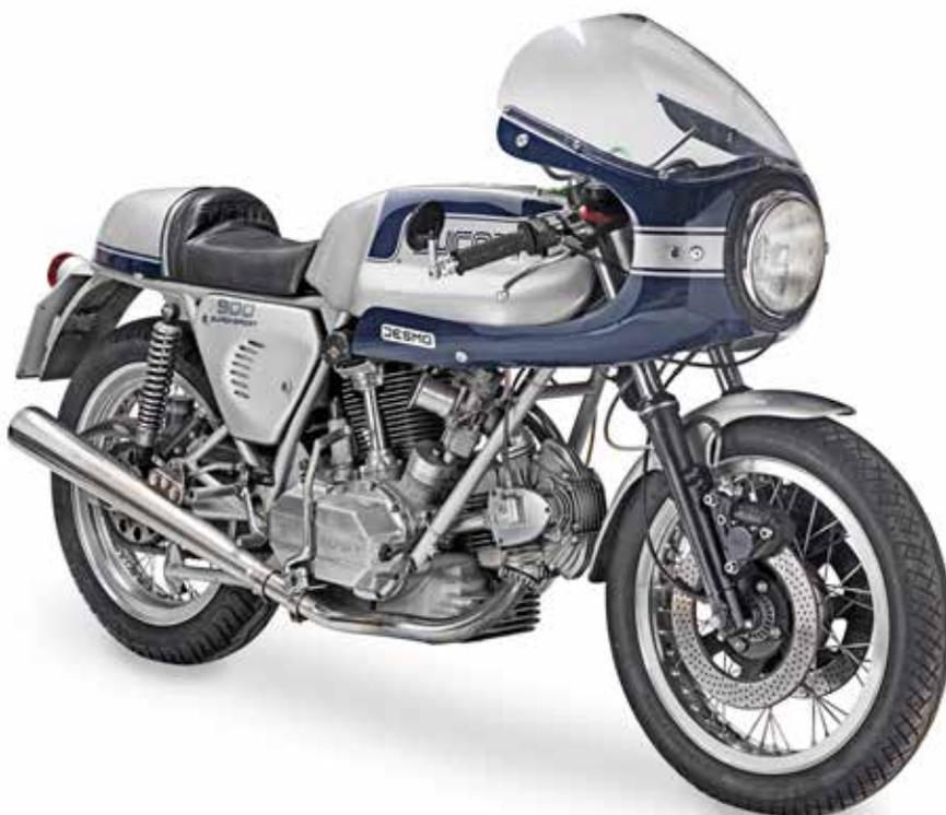
Ducati's second-generation v-twin engine - the 900cc 'square case' (actual capacity 864cc) - debuted in the 860GT of 1974 and the following year was used to power the new 900SS superbike. The latter was styled like the original 750SS that had been developed from Paul Smart's 1972 Imola winner. (The 750SS continued in this new 'square case' guise, though almost all of these smaller, second-generation models were destined for the Italian market).
