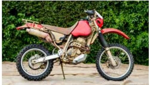
Used for military missions with the SAS. The XL250 is fitted with a 250cc 4 stroke engine. Battle scared green wings, this motorcycle has been well maintained and is running and riding well.
