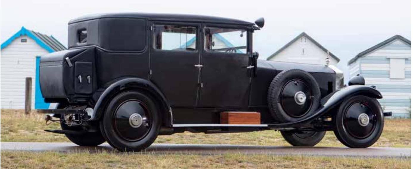
Once the frame, engine, transmission, and axles had been restored and the car brought to rolling chassis state, a replica of the original Gurney Nutting Weymann-type saloon body was fabricated using period photographs as guide. A photograph of '14RF' carrying its original Gurney Nutting body may be found on page 63 of *Rolls-Royce The Derby Phantoms* by Lawrence Dalton.
