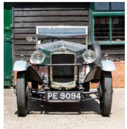
As first conceived, the Frazer Nash chassis employed quarter-elliptic springing, rack-and pinion steering and cable-operated brakes on the rear axle only, though four-wheel braking was soon standardised. The Power Plus 1.5-litre overhead-valve four-cylinder engine was used for the first dozen-or-so cars before the similar-size sidevalve Anzani 4000 series was standardised in 1925.
