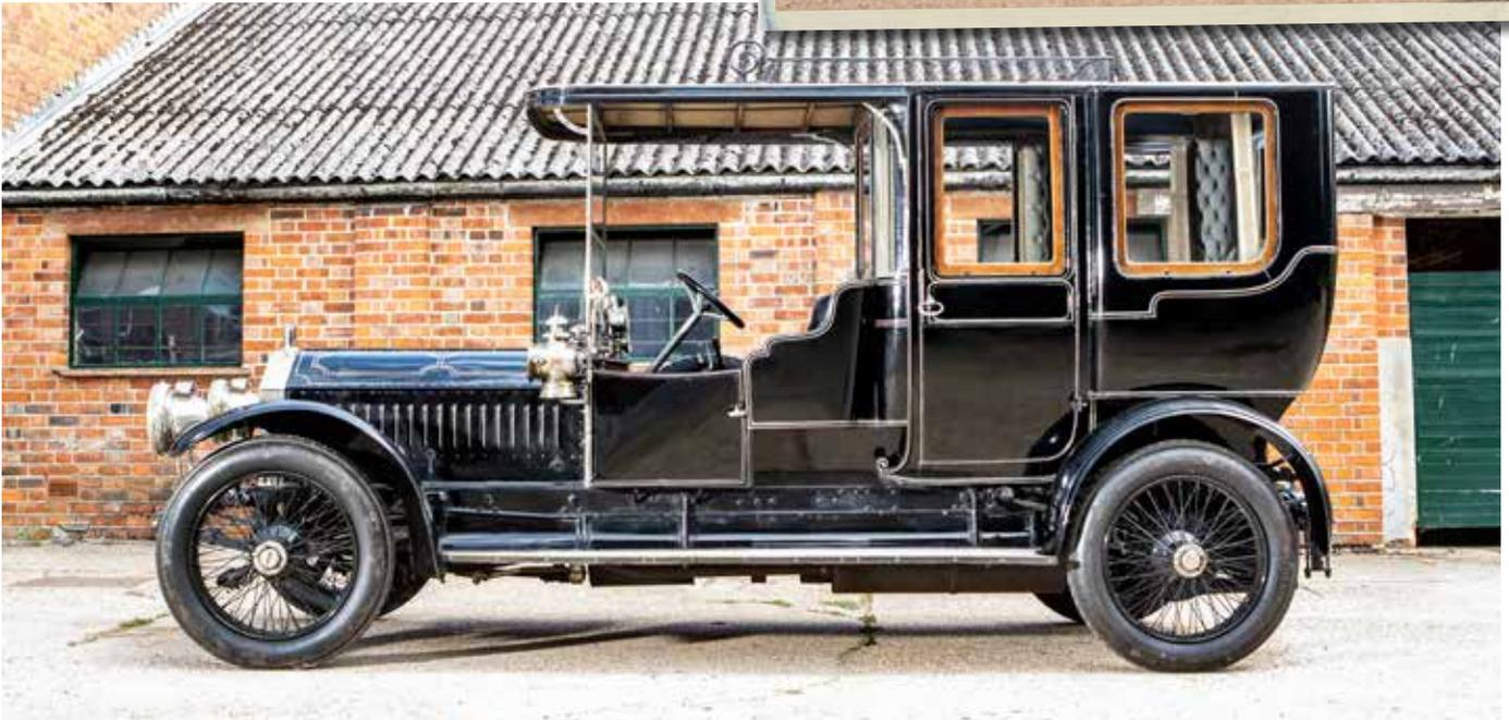
All mechanical work on the chassis and running gear was entrusted to Arthur Archer of Great Dunmow, Essex, who also reproduced the fuel tank and exhaust system. Wheels were rebuilt, brake shoes and drums replaced, patterns made to cast a new water pump, and the electric telegraph from the passenger compartment to the driver repaired. The silk roller blinds have been replaced.
