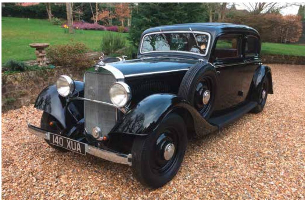
The Mercedes-Benz 200 (W21) was in production from 1933 to 1936, featuring a 2.0-litre straight-six engine, all round independent suspension, and hydraulic brakes. Available in long (3,050mm) and short (2,700mm) wheelbases, this was a 'mid-size luxury car' by the standards of its day.
