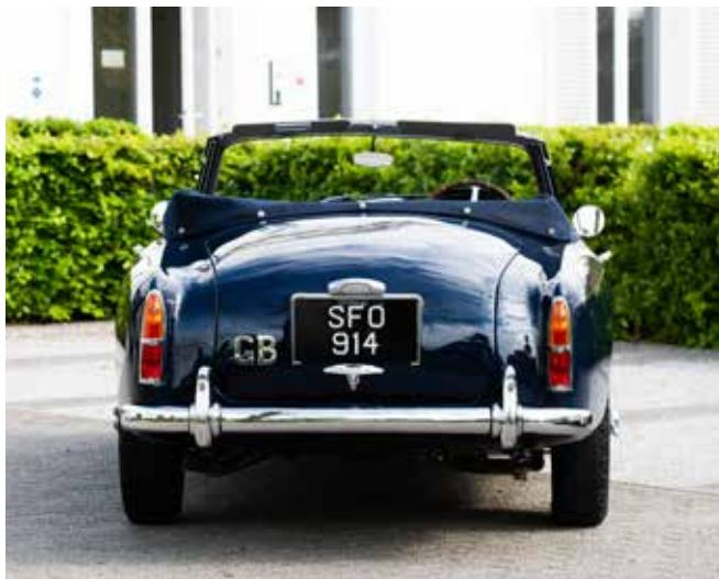
The need to widen the appeal of the already-successful DB2 resulted in the launch in October 1953 of the 2+2 DB2/4. Extensive revisions to the car's rear end arrangements made room for two occasional seats and more luggage, the latter being accessed via a hatchback rear door - one of this now-common feature's earliest applications.
