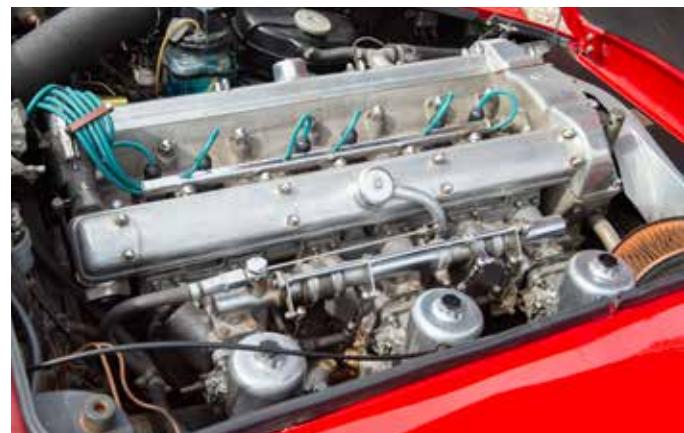
'Racing has played a major part in the development of all Aston Martin engines since Frank Halford designed the original 1.5-litre unit for Bamford & Martin. The 3,995cc 6-cylinder light alloy engine fitted to the DB5 is in all major respects the same as that which powered the 4-litre prototype which ran in the 1962 and 1963 Le Mans 24-Hour races.' – Autocar, 21st May 1965.
