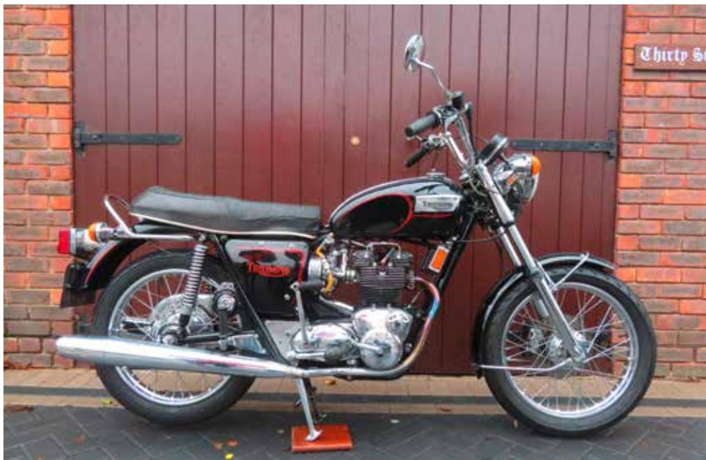
Launched in 1969, the BSA-Triumph 750cc triples were based on the existing Triumph 500cc twin-cylinder engine, being in essence a 'Tiger-and-a-half'. Differences between the Triumph Trident and BSA Rocket 3 were more than just cosmetic: the two models used different frames and in BSA guise the motor featured an inclined cylinder block. Only the Trident survived the group's collapse in 1972, continuing as the five-speed T150V and later the T160 (using the inclined engine).
