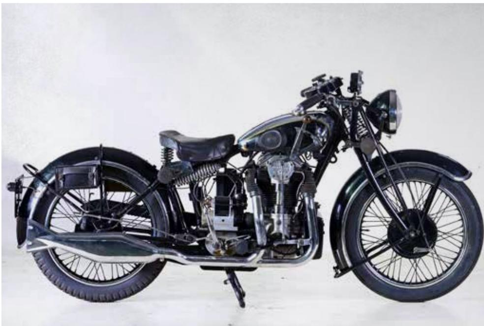
Reviewing the v-four Silver Hawk at its launch in the autumn of 1930, Motor Cycling stated that this exciting overhead-camshaft model was 'designed primarily to give really high speed, and to give this speed with silence and the added safety of a spring frame'.
