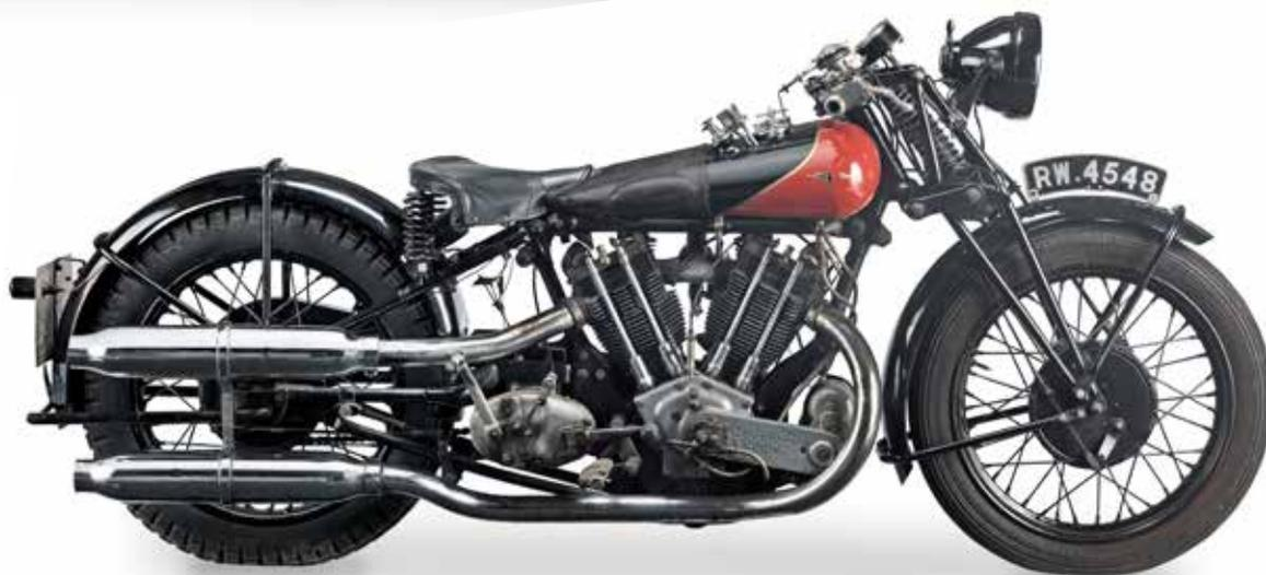
In 1926 the sidevalve version was joined by a new and even faster overhead-valve engine Flying-8, again JAP powered. Motor Cycling concluded its test of the OHV Flying-8 thus: 'We have no hesitation in recommending the latest Coventry-Eagle as a high-quality machine, capable of the most satisfactory road performance both as regards speed and flexibility.' And that, lest we forget, was with a sidecar attached.
