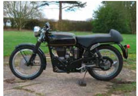
Introduced in 1956, the Venom sports roadster was derived from the touring MSS. The latter had disappeared from the range in 1948, reappearing in 1954 with a new swinging-arm frame and telescopic fork. The engine too was up-dated, changing to 'square' bore and stroke dimensions of 86x86mm and gaining an alloy cylinder barrel and 'head. Engine development pursued as part of the scrambles programme bore fruit in 1956 in the shape of the high-performance Venom and its 350cc sibling, the Viper.
