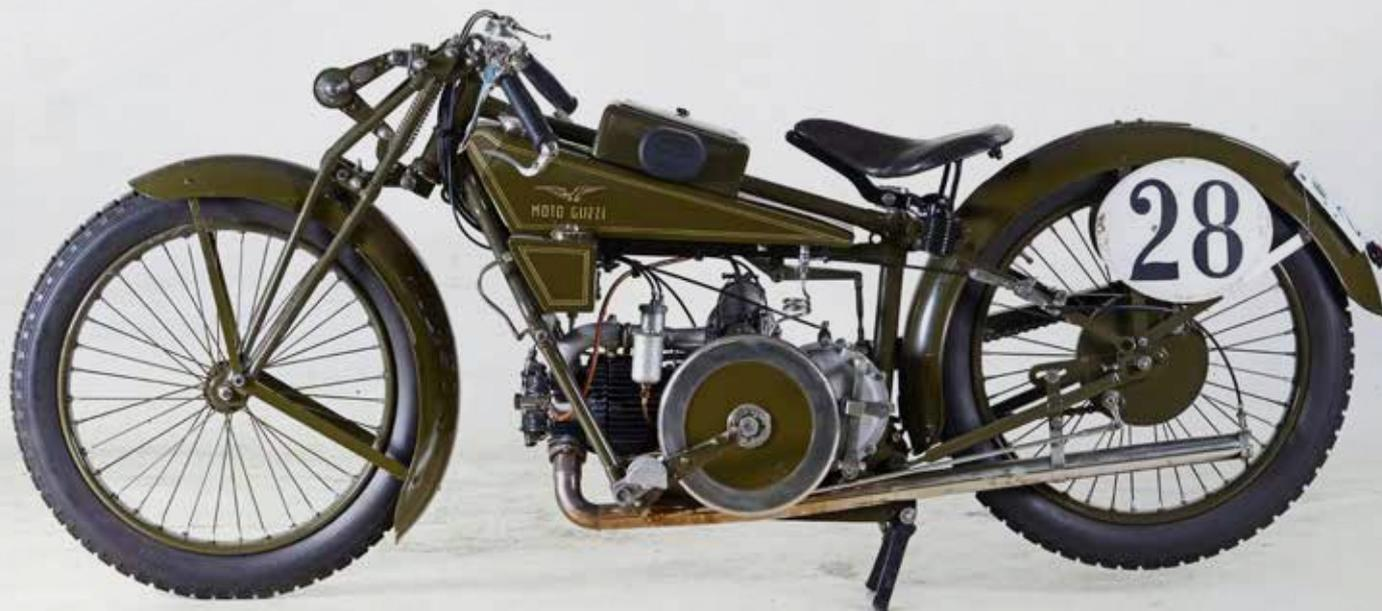
Weighing 290lbs and producing 8bhp, the Normale was good for around 50mph flat out. Although not intended for competition, the Normale was raced by the works prior to the arrival of the purpose-built Corsa 2V for 1923, winning the prestigious Targa Florio endurance classic in 1922. A Tipo Sport spin-off with more powerful engine was catalogued for the first time the following year.
