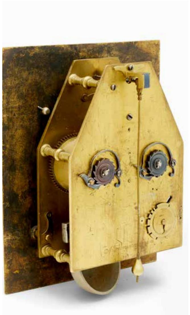
As described by Dawson et al., the movement was originally of two-day duration and later converted to eight days by reversing the barrels and inserting intermediate wheels. The clock is significant because very few short duration clocks have survived from this period. As a practical matter, eight day clocks would have been favored over ones of shorter duration.
