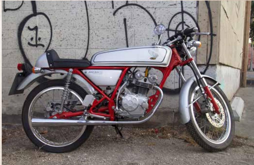
A modern homage to Honda's early Grand Prix road race bikes, two editions featuring race-only 50cc Honda motors with double-overhead camshafts and a 14,500-rpm redline is a masterpiece in miniature.
