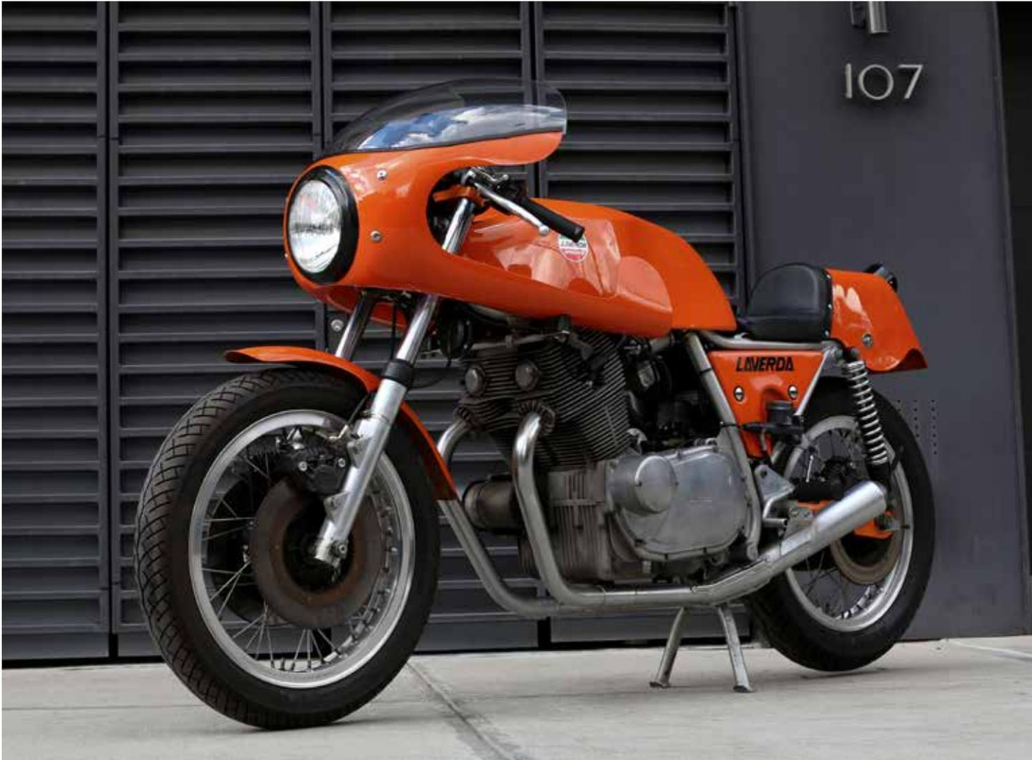
Two of the most significant updates for 1974 was the pair of Dell'Orto PHB 36 carburetors, without accelerator pumps, and twin-bleed Brembo F08 callipers with twin front discs, and a single rear disc on an Elektron hub. A racing two-into-one megaphone (as on this example) accentuated the lean race replica profile, and the claimed power for the 1974 750 SFC was 75 horsepower at 7,500 rpm. The right-side gear shift remained as did Borrani rims and Ceriani suspension front and back.
