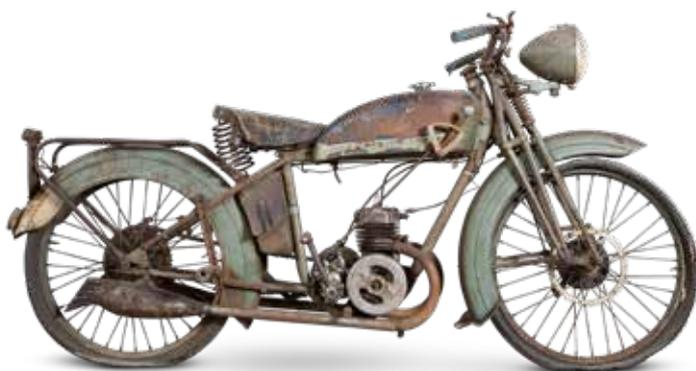
Possibly retaining some original paintwork, this machine is an excellent prospect for restoration. Fitted with a three-speed gearbox and lights, this twin exhaust port two-stroke has a speedometer drive gear to the front wheel, but no speedometer affixed. The engine turns. There are no documents or keys present. Offered strictly as viewed, for restoration, prospective bidders should satisfy themselves as to the completeness, or otherwise, of this lot.
