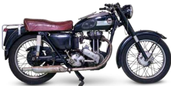
This exhibit is an older restoration, now deteriorating. The rocker boxes are loose, and no rocker oil feeds are fitted. The engine turns over and the speedometer displays 23,725 kms on the odometer. There are no documents, and no key is present. Offered strictly as viewed, for re-commissioning or restoration, prospective bidders should satisfy themselves as to the condition and completeness, or otherwise, of this lot.
