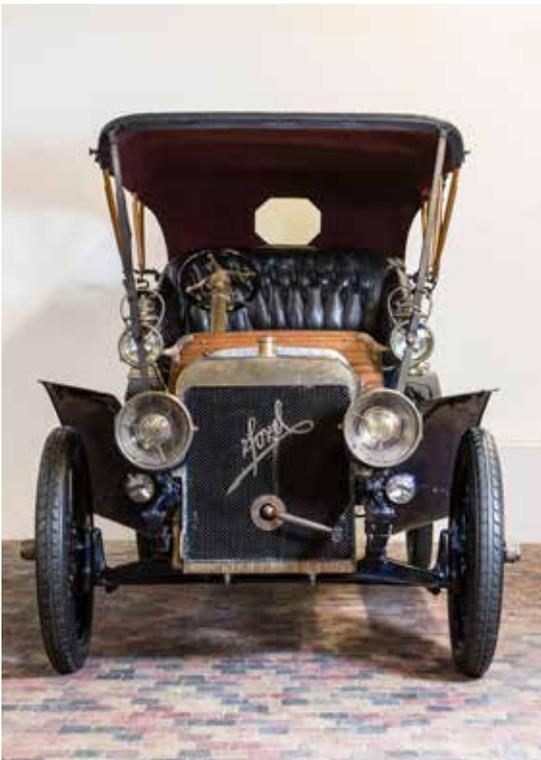
Carlton Pate has kindly provided the specific information that he has on this car, stating that it is an example of the early pattern 4-inch deep frame model, and is fitted with Kristoff transmission, Stromberg glass bowl carburetor, aluminium blade fan and two coil boxes, all signifying its 1906 year. Other detail features which draw the eye are its tiny diagonal Ford script across the radiator, and the large Gray & Davis headlamps as well as their matched sides on the dashboard.
