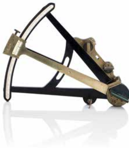
765 AN EARLY 19TH CENTURY 11IN RADIUS EBONY Y OCTANT Y OCTANT Φ Reading from -2 to 100 degrees on the ivory scale, for full description see Bonhams.com, 30cm wide, 8cm deep, 36cm high (11 1/2in wide, 3in deep, 14in high) £300 - 500 €340 - 570
