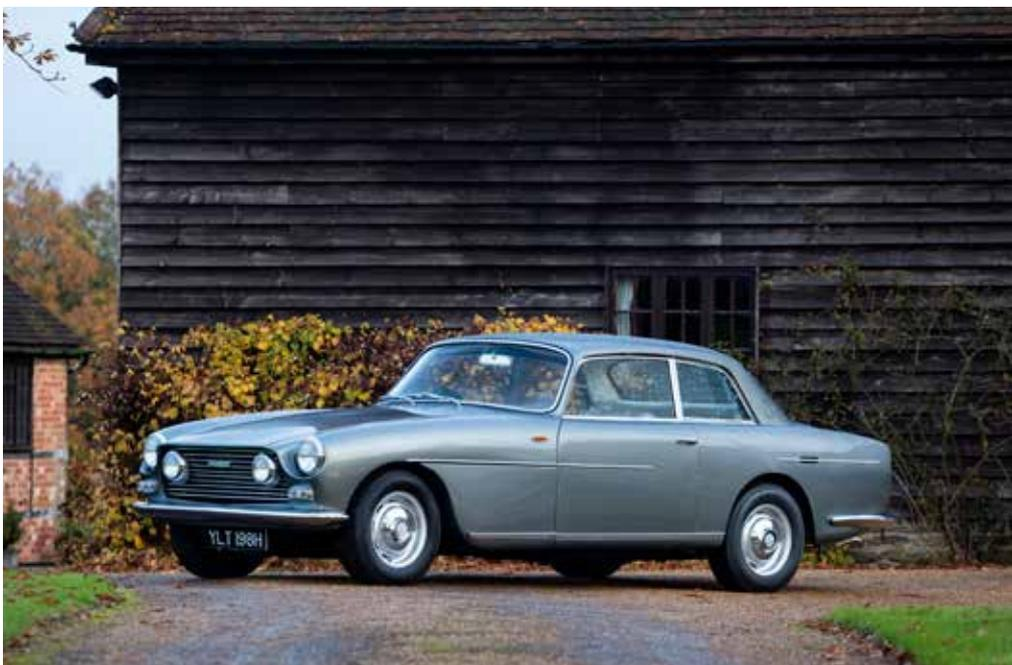
For the 411, introduced at the 1969 Earls Court Motor Show, Bristol continued with Chrysler V8 engines but specified the 6.3-litre unit that produced 335bhp, an increase of some 85 horsepower over the preceding '5.1'. There was a commensurate improvement in performance. With a maximum speed of 140mph and a 0-60mph time of 6.9 seconds, the Bristol 411 was hailed by *Autosport's* John Bolster as 'The fastest true four seat touring car in the world'.
