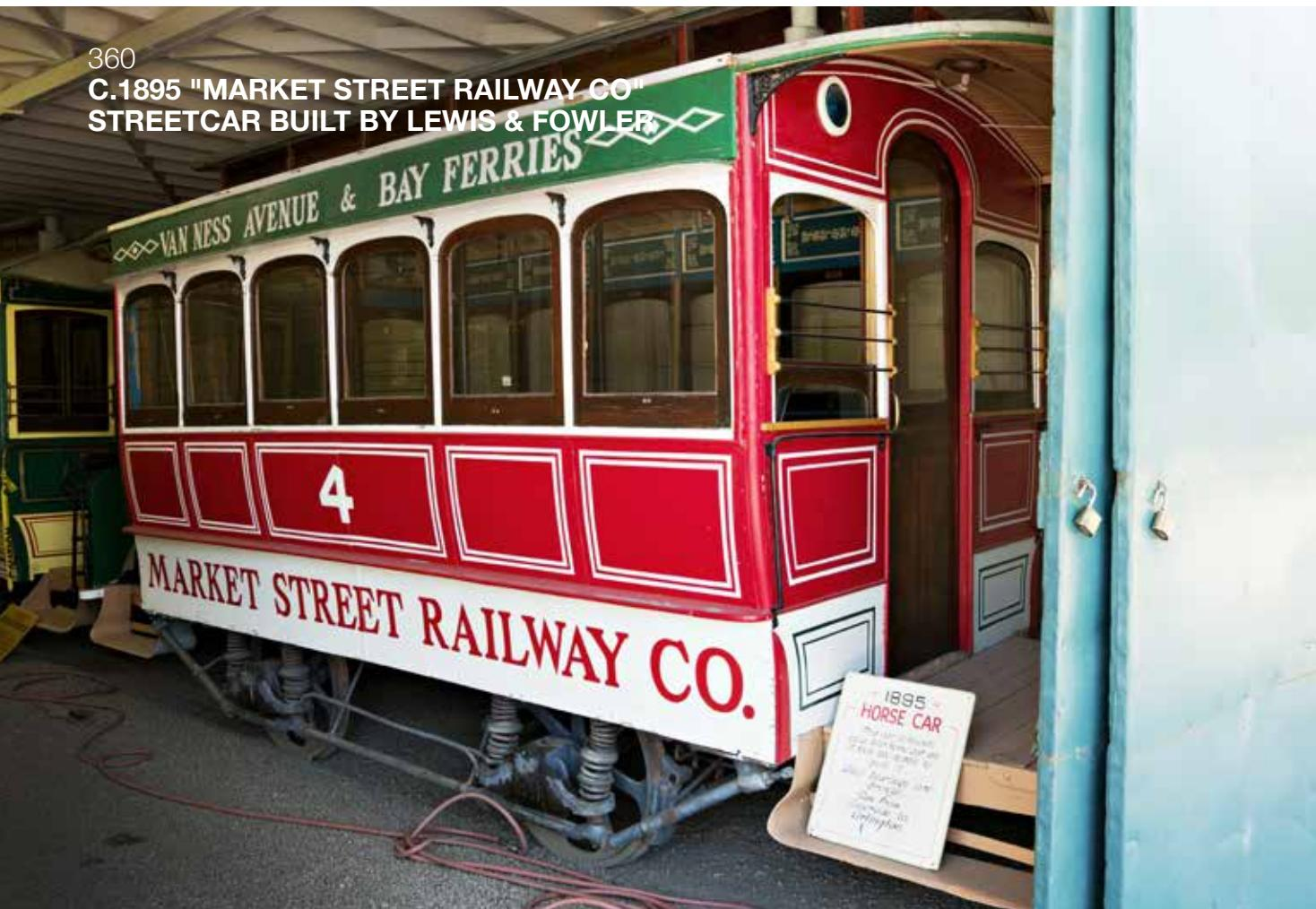
Configured as a fully enclosed vehicle, designed to be pulled by two horses. The streetcar is liveried for the Market Street Railway Co. and destinations of Van Ness Avenue and Bay Ferries.
