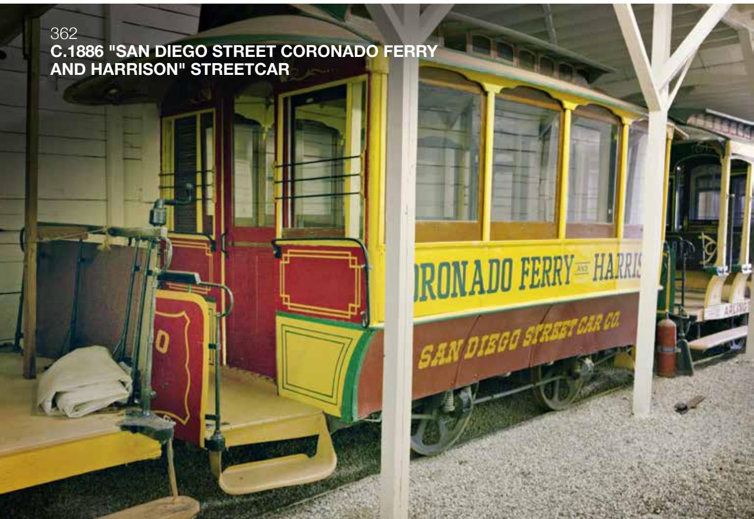
Configured as a fully enclosed vehicle, designed to be pulled by one horse. The streetcar is liveried for the San Diego Street Car Co. and for the destinations of Coronado Ferry and Harrison.
