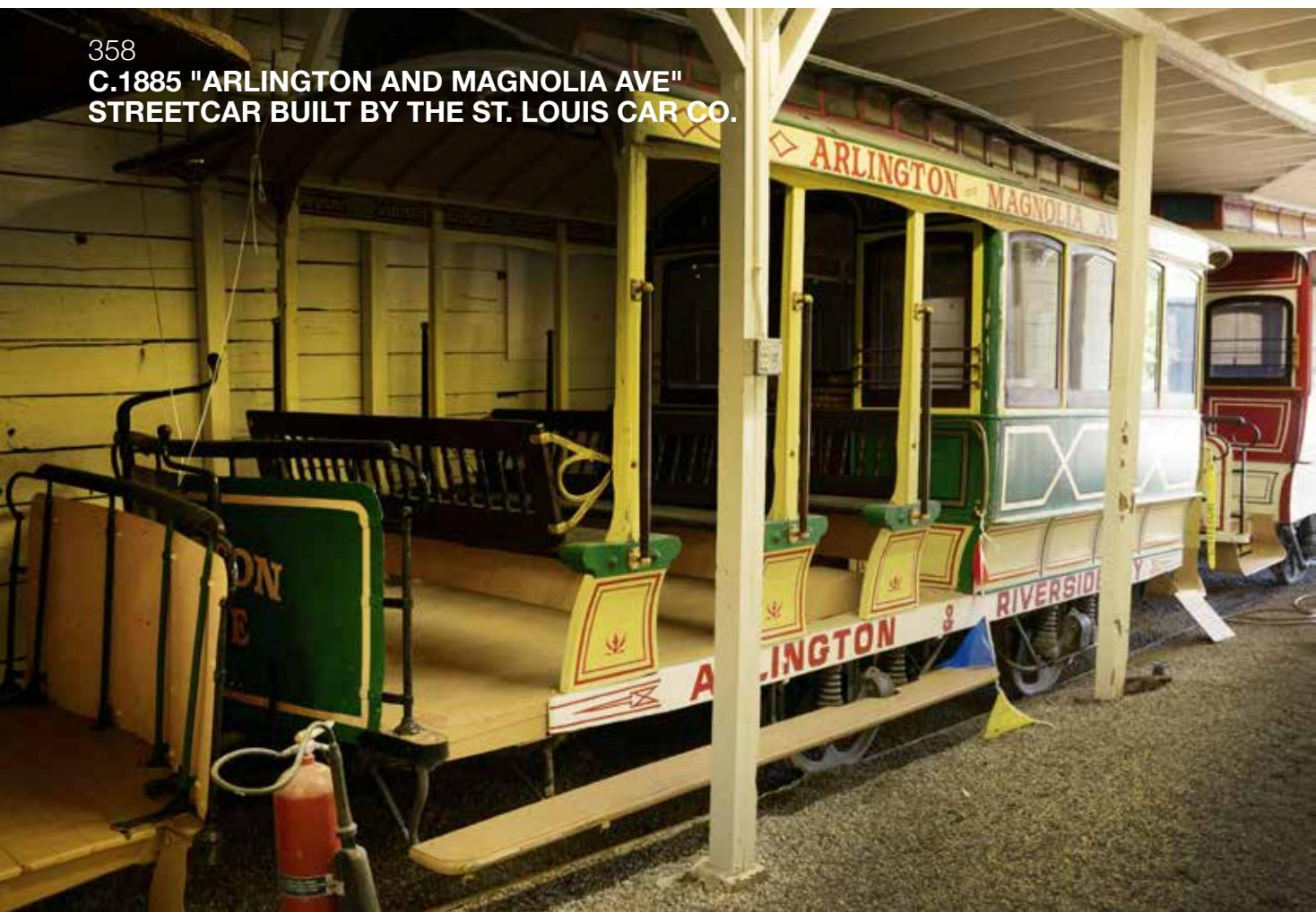
Configured as part open, part enclosed vehicle, designed to be pulled by two horses. This car is believed to have been run on the Riverside & Arlington Railway Company Line and is liveried for Arlington and Magnolia Avenues.
