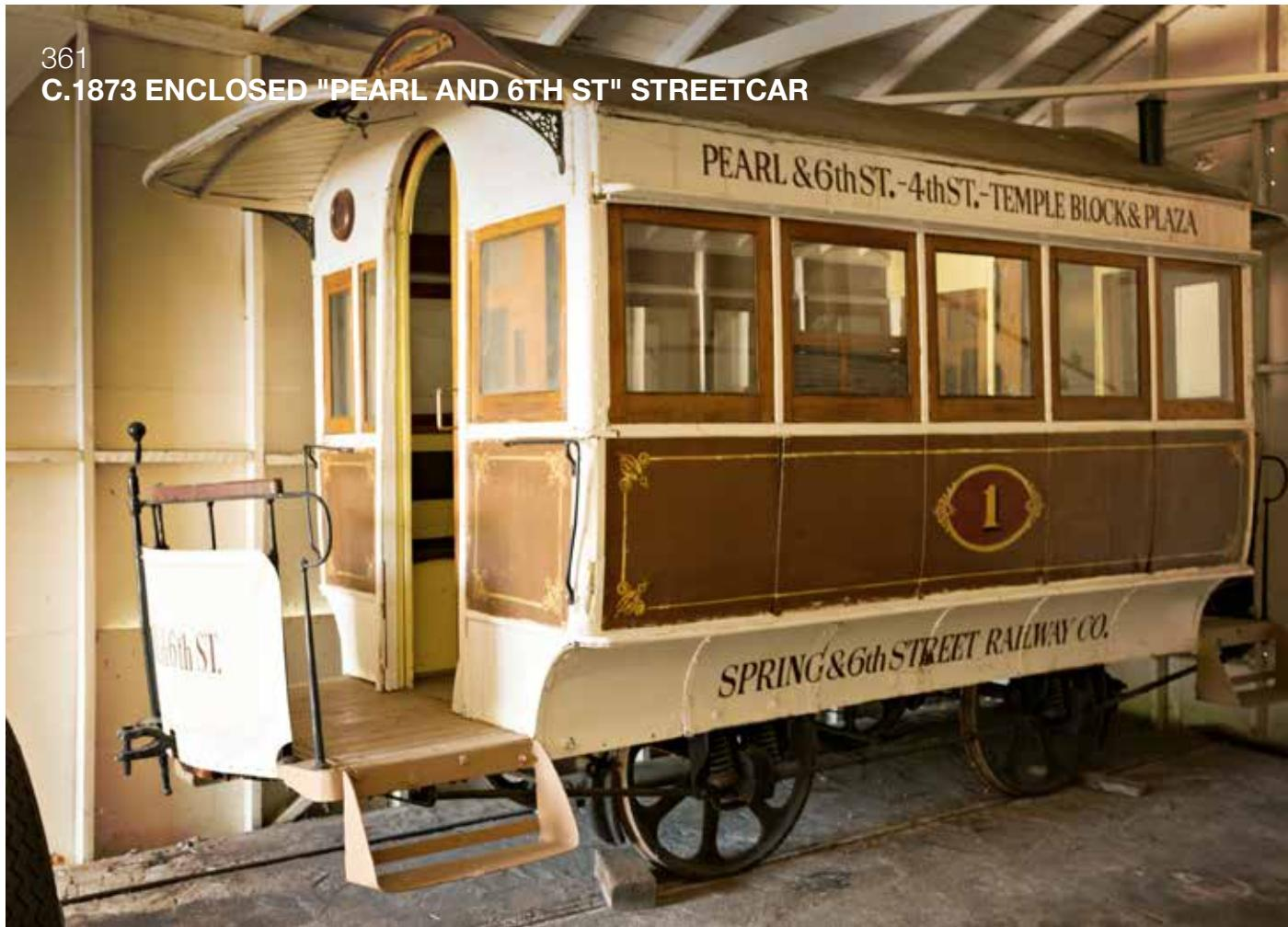
Configured as fully enclosed vehicle, designed to be pulled by one horses. The streetcars is liveried for the Los Angeles based Spring and 6th Street Railway Co. and for the destinations of Pearl & 6th Street. - 4th St. - Temple Block & Plaza.
