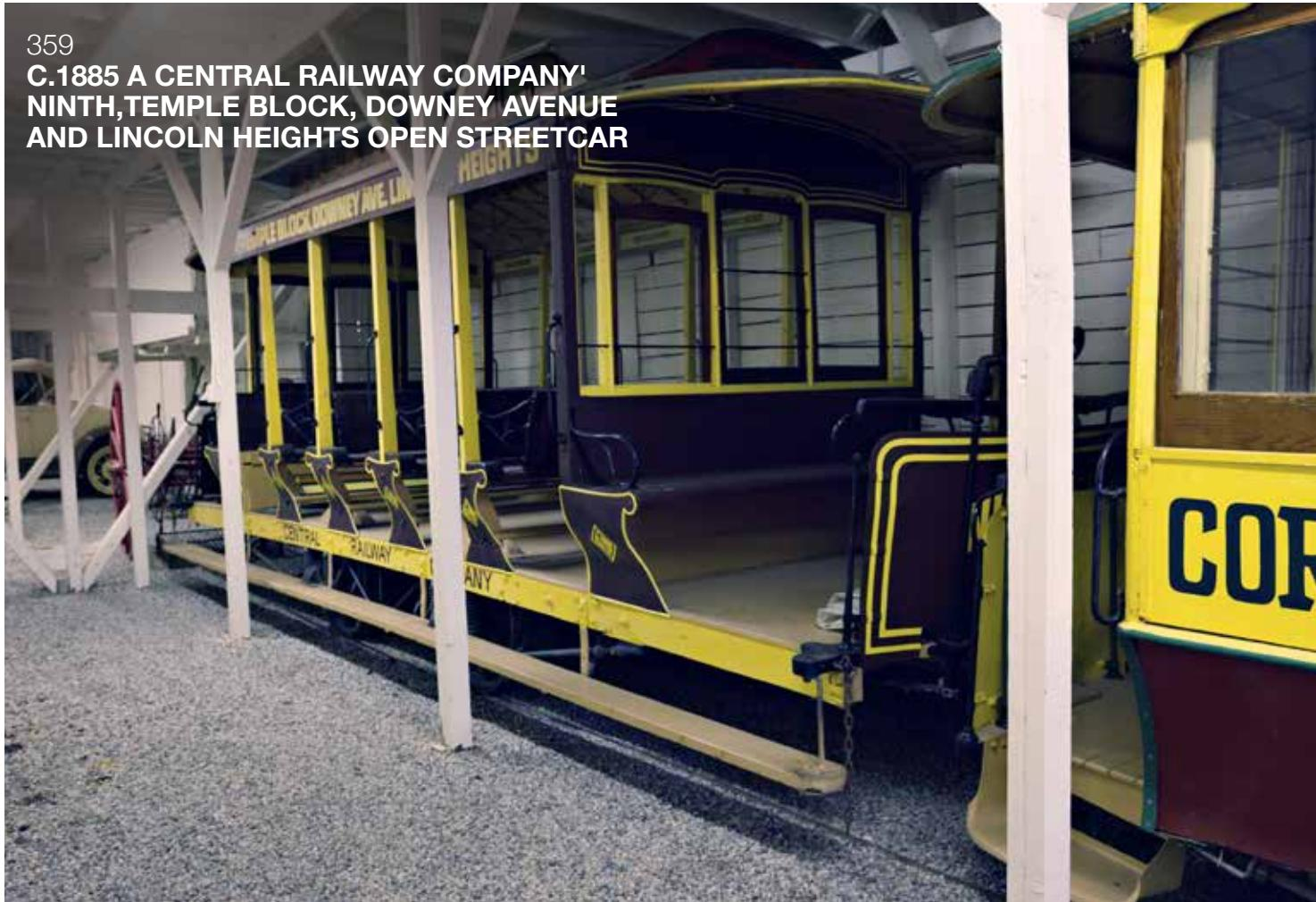
Configured as an open sided vehicle, designed to be pulled by two horses. This streetcar is liveried for the Los Angeles based Central Railway Company, and for destinations of Ninth, Temple Block, Downey Avenue and Lincoln Heights.
