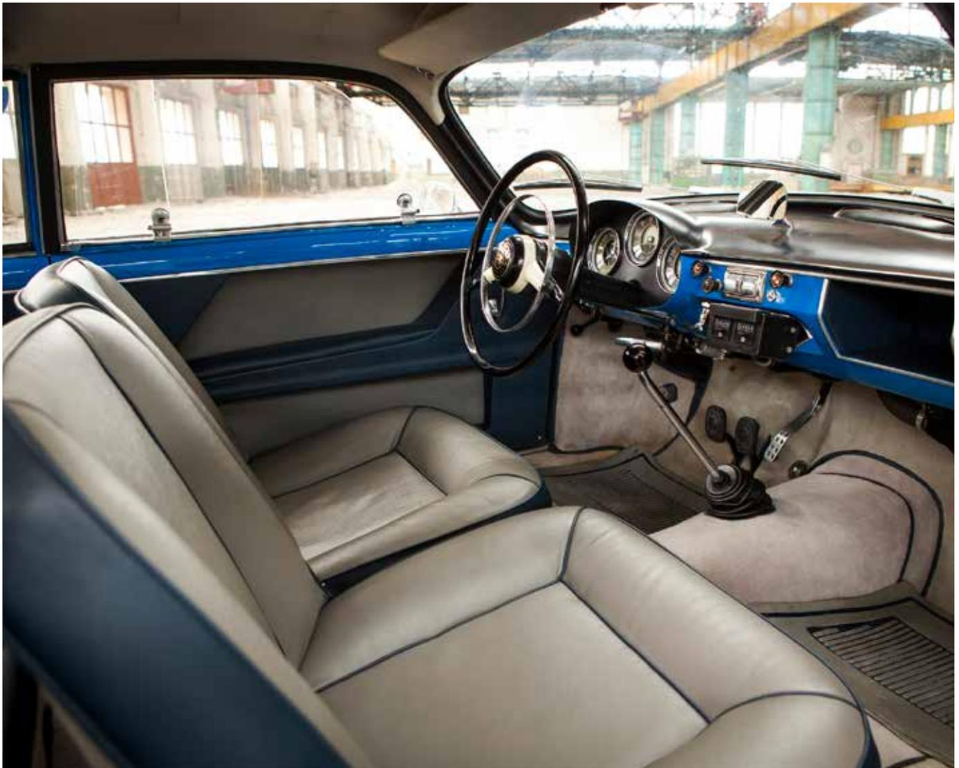
There was no glove compartment cover, no sun visors, and no rear seat. The Veloce seats were thinner, albeit foam-padded, and mounted on a delicate tubular frame. A central gearshift was employed instead of the column-mounted gearshift.
