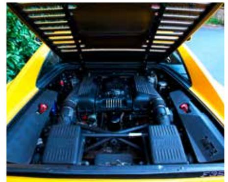
A six-speed gearbox, mounted transversely behind the longitudinally disposed engine, ensured a sufficiency of ratios to keep the motor on the boil whatever the situation.
