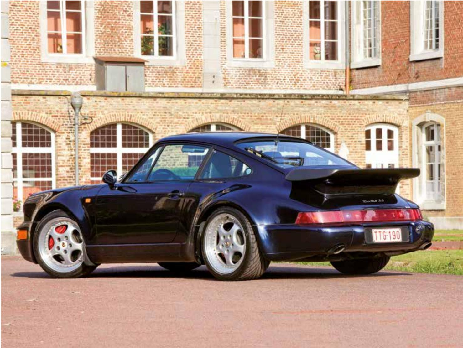
In October 1992 the Turbo received the 3.6-litre M64/50 engine, which in 'blown' form now produced a mighty 360bhp. Along with the raised maximum power output came a welcome increase in torque, addressing the 3.3-litre car's lack of off-boost acceleration. One of the most expensive models in the Porsche range, the 3.6-litre Turbo was produced in limited numbers, only some 1,400-or-so being completed out of a total Type 964 production run of more than 62,000 units.
