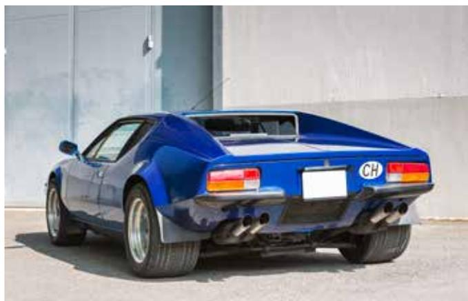
Having established himself as a serious automobile manufacturer with the Mangusta coupé, Alejandro De Tomaso commissioned Lamborghini designer Gianpaolo Dallara to produce the chassis for his new mid-engined supercar, the Pantera. Dallara opted for unitary construction for the steel chassis/body - abandoning the Mangusta's backbone frame - and competition-specification double wishbone/coil-spring suspension all round.
