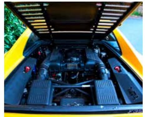
A six-speed gearbox, mounted transversely behind the longitudinally disposed engine, ensured a sufficiency of ratios to keep the motor on the boil whatever the situation.
