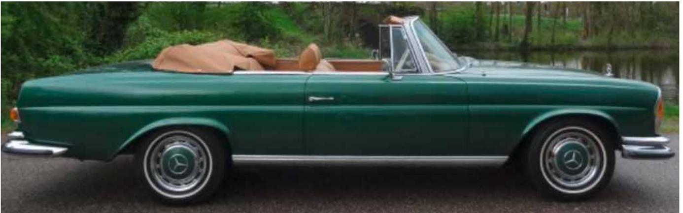
The compact but sturdy engine was capable of moving this big 4/5-seater to 100 kilometres per hour in under 10 seconds, and offered a top speed in excess of 200km/h, a substantial improvement on the six-cylinder version's figures. Large vacuum-assisted disc brakes at each corner allowed the driver to slow with ease, and handling was described as very comfortable, thanks to its coil-sprung independent suspension.
