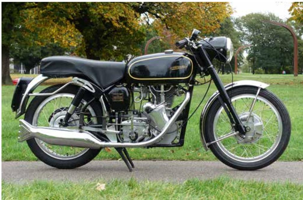
Introduced in 1956, the Venom sports roadster was derived from the touring MSS. The latter had disappeared from the range in 1948, reappearing in 1954 with a new swinging-arm frame and telescopic fork. The engine too was up-dated, changing to 'square' bore and stroke dimensions of 86x86mm and gaining an alloy cylinder barrel and 'head. Engine development pursued as part of the scrambles programme bore fruit in 1956 in the shape of the high-performance Venom and its 350cc sibling, the Viper.
