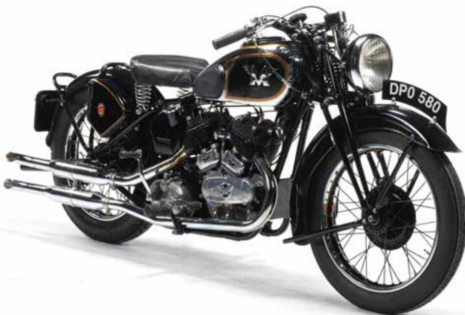
Offered here is a late 1937 (1938 model) Matchless Model X; it is the revised version having a longer wheelbase, which was re-launched as a sports tourer. Brough Superior used this engine in the SS80 and also (in overhead-valve form) in the SS100.
