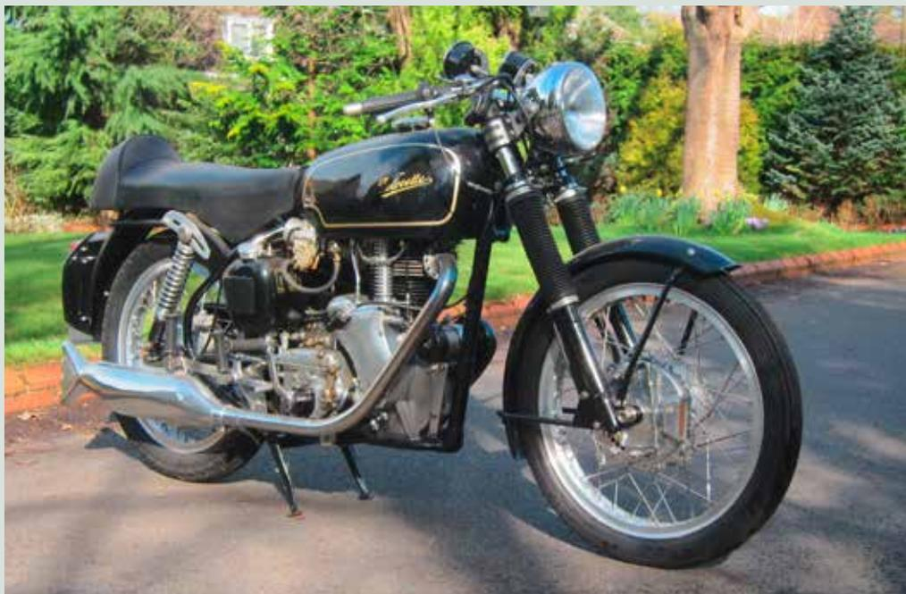
'Prestige machine of the pushrod range was the Venom Thrupton 500. It incorporated all the accumulated experience gained in the years the Venom Clubman has been raced in long-distance events, plus the development of the 12 and 24-hour record breaker.' – C E A 'Titch' Allen, The Velocette Saga.
