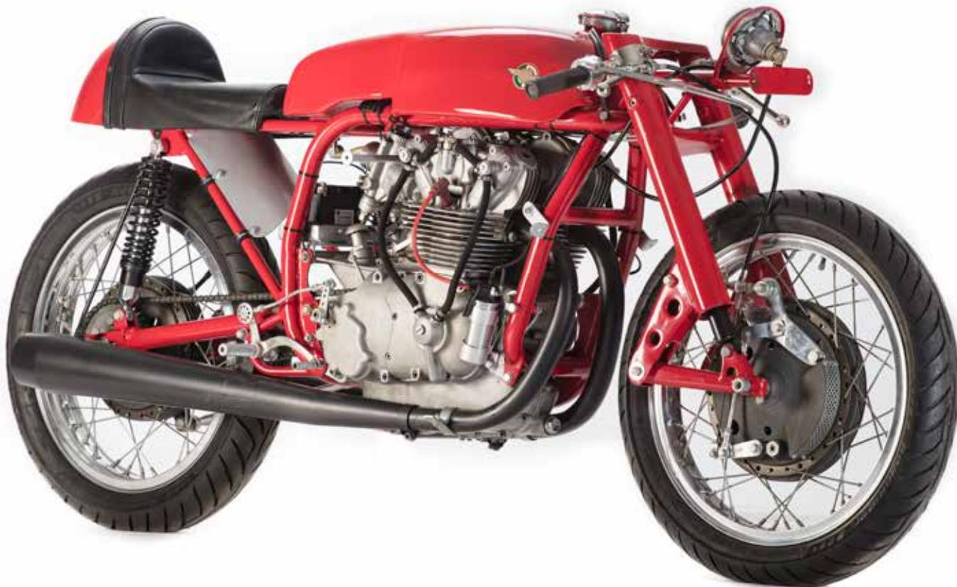
Commissioned by John Surtees circa 1961, the ultra-rare machine offered here incorporates an ex-works Ducati desmodromic twin-cylinder engine, which is housed in a bespoke frame fabricated by maestro frame-maker, Ken Sprayson. It is one of a pair, the other being a '350', which were built for Surtees using engines taken from machines supplied by Ducati for the use of Mike Hailwood.
