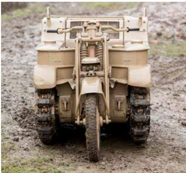
The Kettenrad was typical of vehicles designed and manufactured for the German Wehrmacht during WW2: innovative, well made, and generally superior to equipment used by their enemies. Designated 'SdKfz 2' by the German Army, the Kettenrad was an ingenious half motorcycle, half tracked vehicle, hence its name – 'ketten' meaning tracks, 'krad' meaning Krafttrad or motorcycle.
