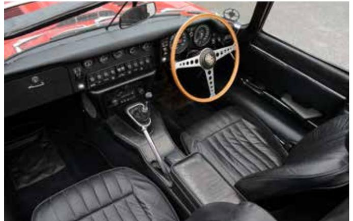
In addition, enlarged side and rear lights were adopted while a thickened front bumper centre section bridged a larger radiator intake. Interior changes included a collapsible steering column and rocker switches in place of the earlier toggles.
