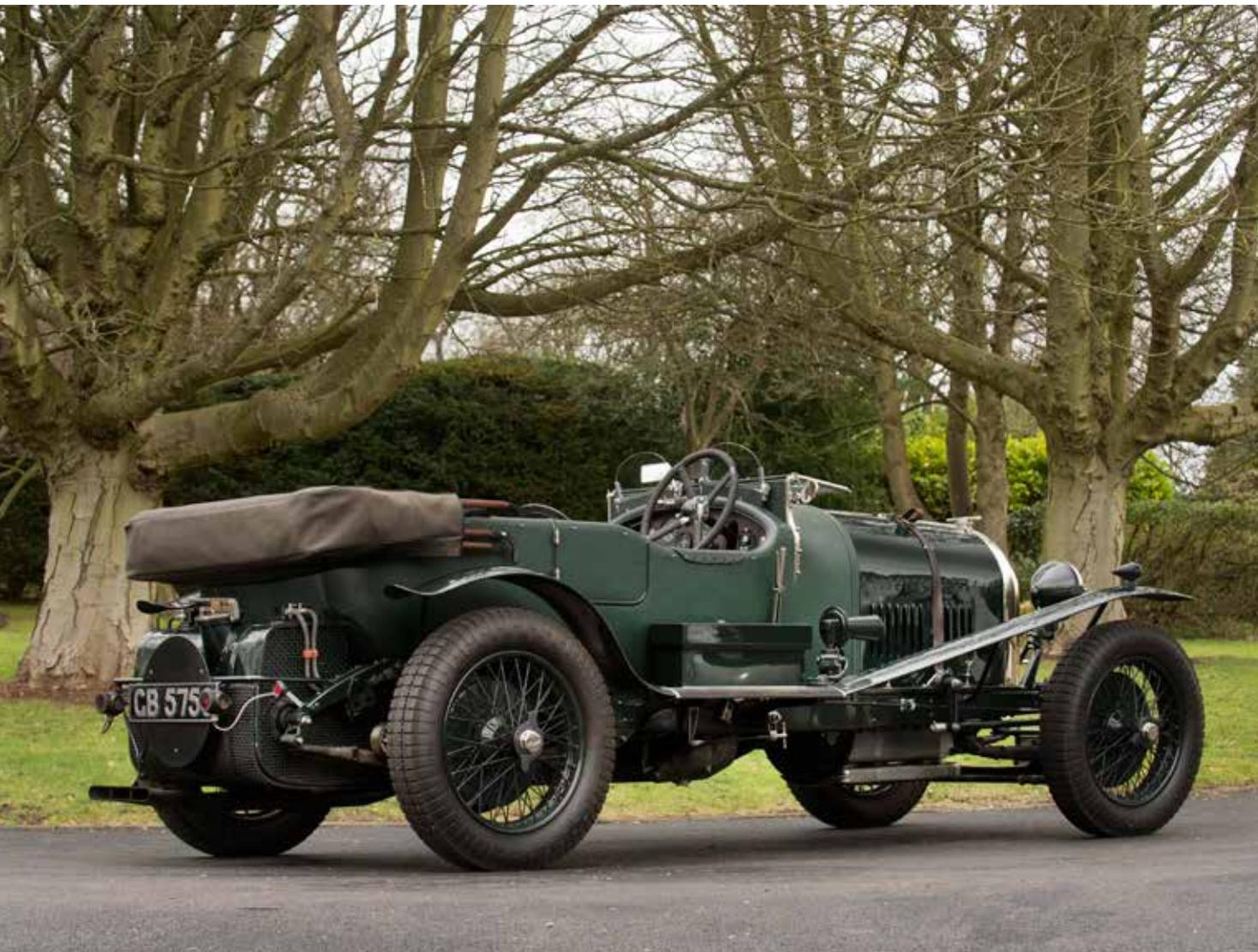
The car has correct finned brake drums at the front and plain drums at the rear. These were machined true. The Perrot shafts were overhauled and the pedal shaft re-metalled and ground to the correct dimensions, and every joint and moving part in the system re-metalled as required or re-bushed with new pins to eliminate all wear. New brake linings were fitted together with new André Hartford shock absorbers front and rear.
