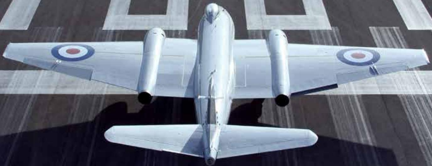
The English Electric Canberra is a British jet-powered bomber manufactured in large numbers throughout the 1950s. The Canberra could fly at a far higher altitude than any other bomber during the 1950s and went on to set a world altitude record of 70,310 ft in 1957. Due to its ability to evade the early jet interceptors and its significant performance advancement over contemporary piston-engined bombers, the Canberra was a popular export product and served with air forces of many nations.
