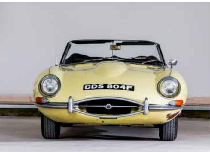
Launched in October 1964, the 4.2-litre version of Jaguar's sensational E-Type sports car brought with it a more user-friendly all-synchromesh gearbox and a superior Lockheed brake servo along with the bigger, torquier engine. Top speed remained the same at around 150mph, the main performance gain resulting from the larger engine being improved acceleration.
