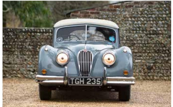
Like its forbear, the XK140 was built in three model types: roadster, coupé and drophead coupé, the latter two offering usefully increased cabin space and occasional rear seats. Outwardly the newcomer was distinguishable by its revised radiator grille, rear lights incorporating flashing indicators, and larger bumpers - the latter adopted to withstand the cut and thrust of urban parking.
