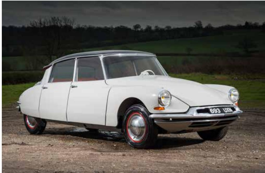
This is a very good example of the revolutionary Citroën DS19 in the form in which it first appeared at the 1955 Paris Auto Show. Besides the famous Hydropneumatic self-levelling suspension, it has the four-speed semi-automatic transmission, power steering and power brakes. It was built in the autumn of 1957 and is among the first 30,000 DS19s built out of a total of 1,456,000.
