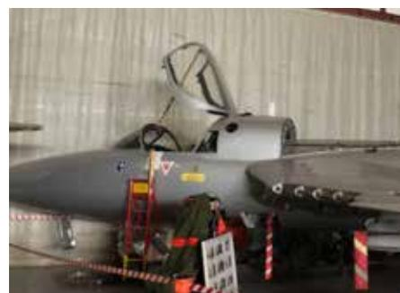
The Hawker Hunter was designed as a single seat fighter with swept wings, variable incidence tailplane (electrically actuated follow-up trim) powered aileron and elevator controls and pressurised cabin, powered by a Rolls-Royce Avon 100 engine. The T7 is a two seat side-by-side trainer/operational version intended for training and conversion operations and is powered by a Rolls-Royce Avon Mk 122 turbine engine.
