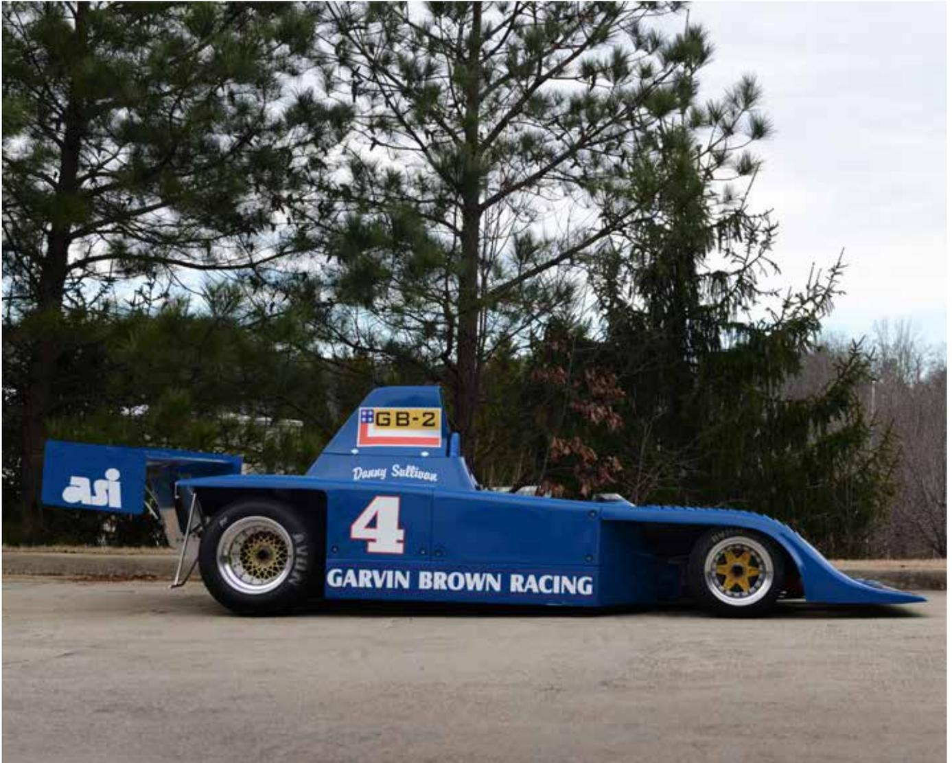
Frisselle decided to fix the problem by hiring master fabricator Jack Smith to construct an entirely new tub (Frissbee chassis #2) of 2024 aluminum and 4130 steel from a design by Trevor Harris. Much of the development concentrated on improving torsional rigidity and the car's aerodynamics, and Harris came up with a number of innovations, including a reverse front underwing that increased downforce and helped stabilize the handling.
