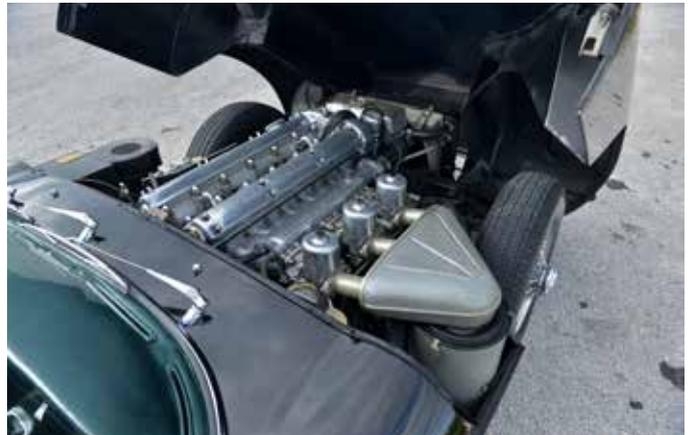
including its matching-numbers 4.2L inline six cylinder with triple SU carburetors, and 4-speed manual gearbox.
