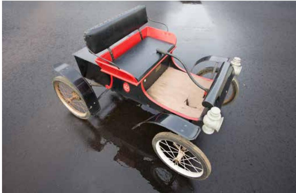
This charming little Oldsmobile was built by Hallock Manufacturing Company of Strasburg Pennsylvania. A four-cycle Clinton engine powers this well made little machine is powered by. It features an automatic clutch and a foot brake. Steering is faithful to the original with the famous central tiller.
