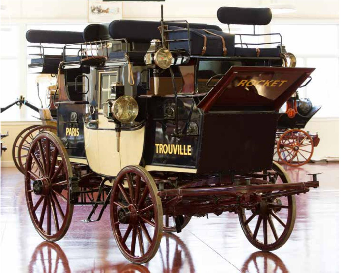
feature is that beneath the rear squab is a formal toilet! The headlining is oil cloth, painted and stained in a wood effect finish. The roof seat cushions, guard and coachman's seats are finished in dark blue cloth also. Between the roof seats is a storage trunk and adorning either side the are two sets of side lamps.
