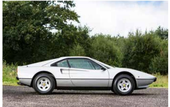
The Ferrari 308 GTB offered here has lighter glass fibre (vetroresina) bodywork and dry-sump lubrication of the very first cars produced, which are the most sought after by enthusiasts today.
