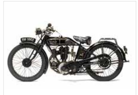
Wars have always spurred on technological development, the rush to produce ever more powerful aero engines in WWI being a case in point, establishing as it did the superiority of overhead valves over the alternatives when high performance was paramount. There had been overhead-valve car and motorcycle engines before 'The Great War', but with the layout's superiority emphatically demonstrated, it did not take long before new OHV designs began appearing on the world's roads in substantial numbers.
