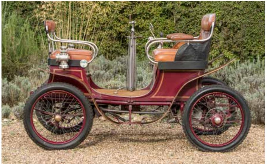
Following the success of its tricycles and quadricycles, the De Dion-Bouton company introduced a new generation of four-wheeled vehicles in 1899 with a rear-mounted engine driving the rear wheels via a train of gears. With the new car came the renowned De Dion rear axle, which would find favour with many makes over the years. Originally powered by a 3½hp engine, it was upgraded with a 4½hp in 1900 and this example has the latter power unit.
