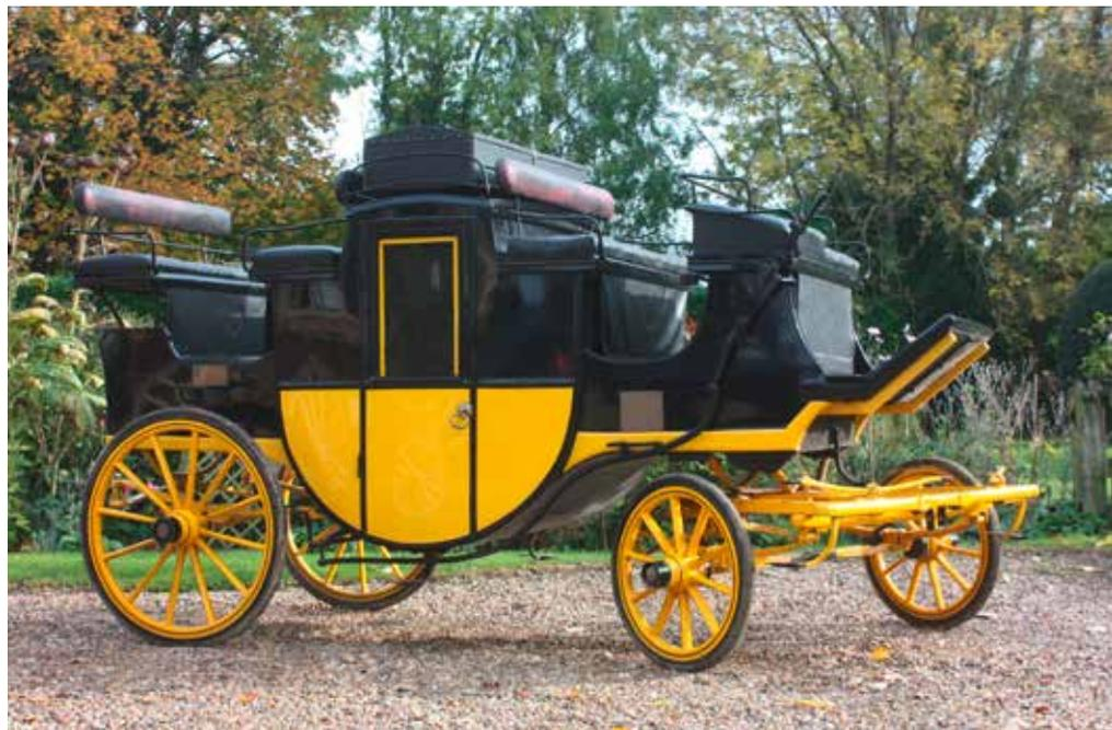
It is not known when this professionally made Pony Drag was constructed, or by whom. It was purchased by the vendor in 1990 and entrusted to specialists Fairbourne Carriages to carry out a refurbishment. Bills on file detail the works, viewing of which is recommended; works included rebuilding wheels, replacing the front axle, repairs to springs, brakes and repairing the wood framing to the coach.
