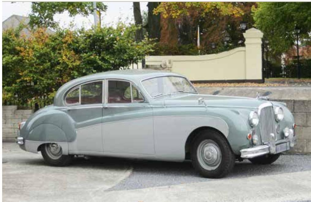
Work on Jaguar's new advanced saloon had been interrupted by the war, and it was not until 1950 that the design saw the light of day as the Mark VII. A considerable improvement on what had gone before, the cruciform-braced chassis featured torsion-bar independent front suspension and all-round hydraulic brakes. The 3.4-litre six-cylinder XK engine had already demonstrated its prowess in the XK120 sports car and proved capable of propelling the Mark VII's not inconsiderable bulk past 100mph.
