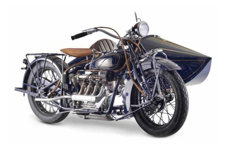
Marketed as the Indian Ace for 1928, the Springfield company's first four-cylinder motorcycle had resulted from its purchase of Ace rights and tooling from Detroit Motors the previous year. The Ace company, although bankrupted twice, had developed a fundamentally sound fourcylinder motorcycle based on William Henderson's original design, and this provided Indian with an opportunity to offer an in-line 'four' with minimal development costs.
