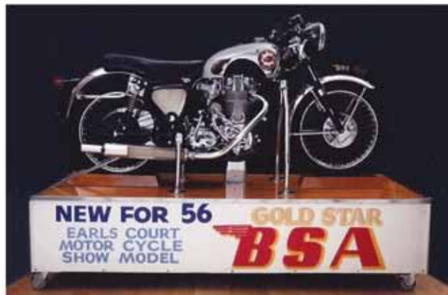
Earls Court Show BSA Gold Star operational cutaway complete motorcycle
