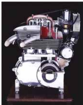
Ariel Square Four cutaway engine
