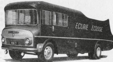
Basis of the new 'Ecurie Ecosse' racing car transporter is the world renowned Commer 7 ton f.c. chassis powered by the phenomenal Rootes diesel engine, a high speed direct injection two-stroke of unsurpassed economy which develops 105 b.h.p. It has an outstanding power/weight ratio and an excellent torque at low speeds.
