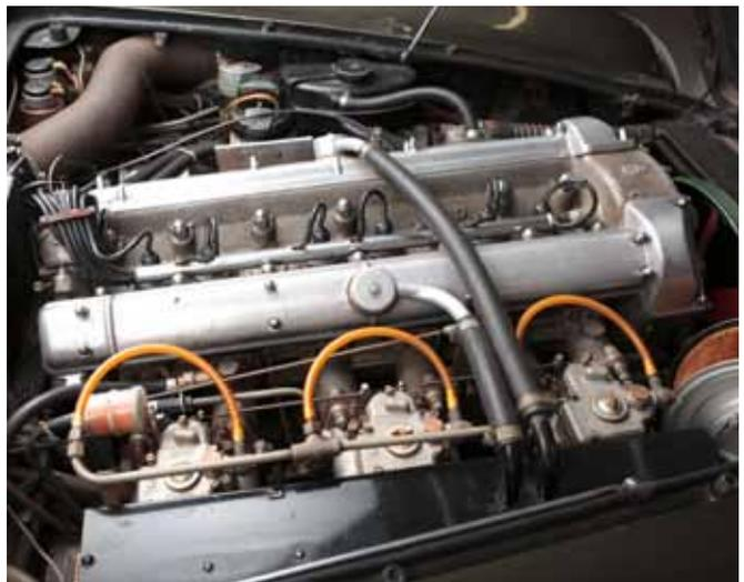
The Tadek Marek-designed six-cylinder engine had been enlarged to 3,995cc for the preceding DB5 and remained unchanged. Power output on triple SU carburetors was 282bhp, rising to 325bhp in Vantage specification. Borg-Warner automatic transmission was offered alongside the standard ZF five-speed gearbox, and for the first time there was optional power-assisted steering.
