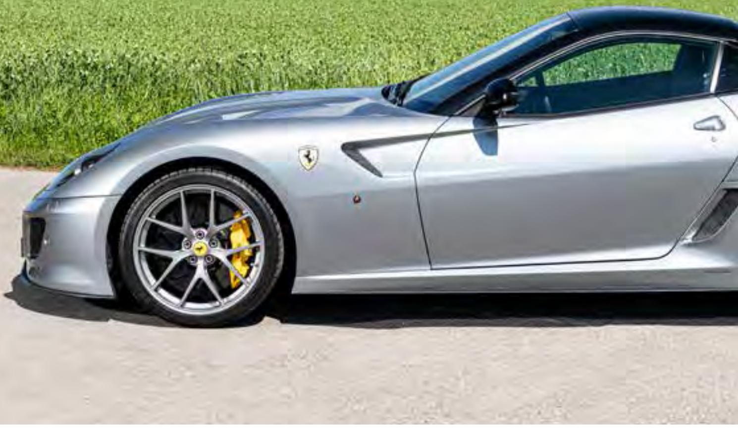
The body's aerodynamics were developed in the wind tunnel, where hours of testing ensured that the minimum of drag was combined with constant downforce regardless of set up, an important consideration in a 200mph road car. Styling details such as the front brake ducts and hot air outlets behind the front wheelarches recalled the great competizione Ferraris of the past while the tail incorporated Ferrari's characteristic twin circular lights.
