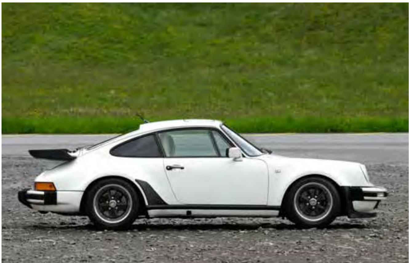
In 1978 the Porsche 911 Turbo's engine was enlarged to 3.3 litres; power increased to 300bhp and the top speed of what was the fastest-accelerating road car of its day went up to 160mph (257km/h). More refined than hitherto yet retaining its high-performance edge, the Porsche 911 Turbo sold in the thousands, becoming the definitive sports car of its age.
