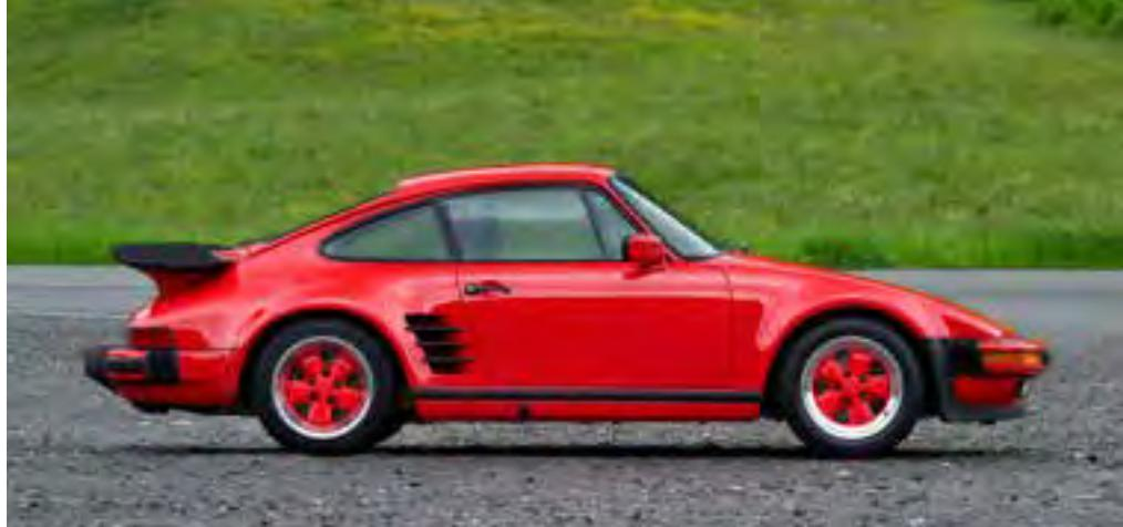
The racing Type 935 version of the Type 930 Turbo pioneered the 'slant' or 'flat' nose. Kremer Racing offered a conversion, as did the factory's own Customer Department from 1981, becoming an official option in 1986.
