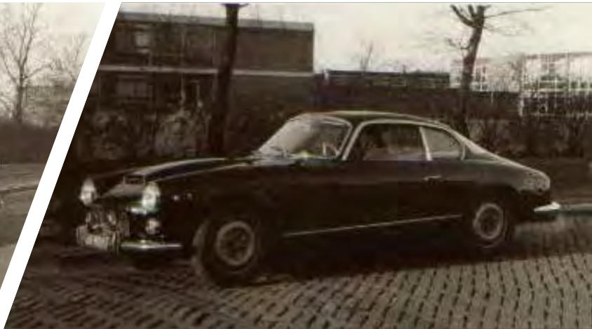
This striking Zagato-bodied Lancia Flaminia Sport features the Milanese styling house's renowned 'double bubble' body form in which low overall lines and a rounded streamlined shape are achieved by the simple but ingenious device of convex head-clearance roof bulges above each front seat.
