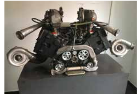
6 1986 FORD COSWORTH F1 1500CC ENGINE PRODUCING 1000 BHP AT 12,200 RPM €10,000 - 15,000 No Reserve
