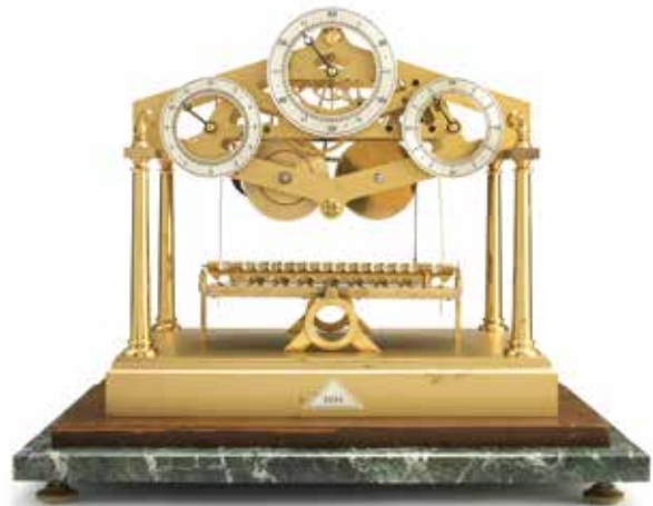
724 A BRASS CONGREVE ROLLING BALL TIMEPIECE TP signed Dent, circa 1970s, the three silvered Arabic chapter rings showing the hours, minutes and seconds, mounted on a pierced lozenge-shaped frame united by four turned pillars, further supported by four turned columns, the substantial single fusee movement with Harrison's maintaining power, the escapement comprising a pivoted runway, the seconds via a roll-over silvered indicator, on a mahogany plinth and marble base with perspex cover the base 49cms wide (2) £1,800 - 2,000 €2,000 - 2,300
