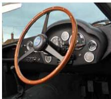
This DB4 Zagato re-creation started life as a standard DB4 sports saloon, chassis number 'DB4/404/R'. It was purchased in 1998 and subsequently completely stripped of every component, and the chassis sent away for sandblasting. On return the car was entrusted to renowned Aston Martin restoration specialists Bodylines of Olney for conversion to DB4GT Zagato specification. The aluminium body was built to lightweight specification with the 'deep nose' considered by many to be the best looking.
