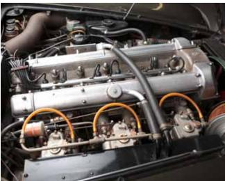
The Tadek Marek-designed six-cylinder engine had been enlarged to 3,995cc for the preceding DB5 and remained unchanged. Power output on triple SU carburettors was 282bhp, rising to 325bhp in Vantage specification. Borg-Warner automatic transmission was offered alongside the standard ZF five-speed gearbox, and for the first time there was optional power-assisted steering.
